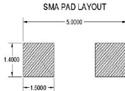
**Mechanical Dimensions SMA (Inches/Millimeters)**
